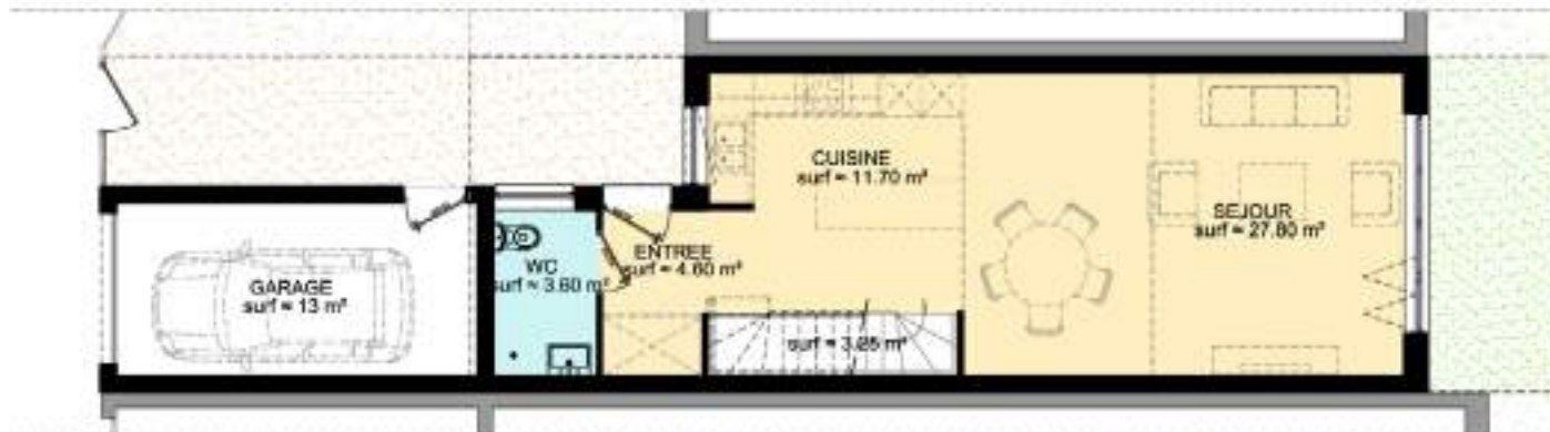
Plan Rez-de-chaussée - Surface = 51 m 2
