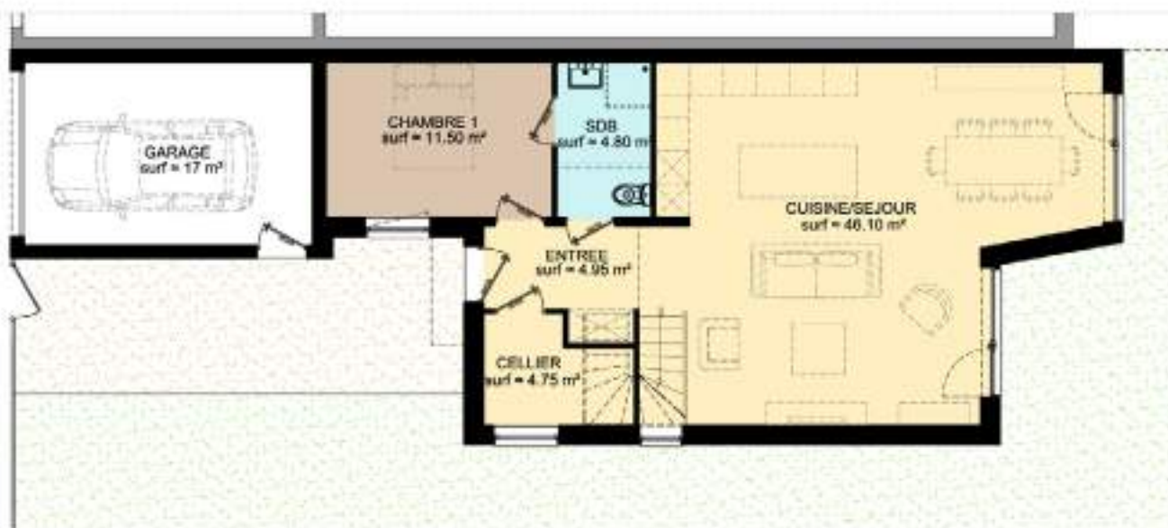
Plan Rez-de-chaussée - Surface = 73 m 2
